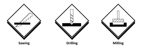
The machining of VEKAPLAN sheets can be done using common tools which are also used for the processing of wood and metal. Basically, you should work at high cutting speed, minor feed and low chipping depth.
