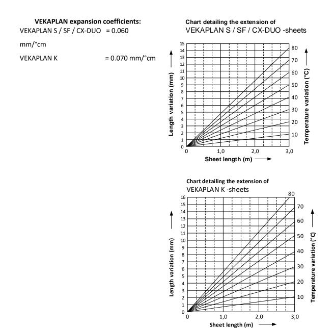
As a general rule, the expansion-related movement in the case of sheet-like components occurs from the centre of the sheet towards its edge. Fixings at the edge area will inhibit such movement leading necessarily to the formation of dents. In order to avoid that effect, appropriate expansion joints, hole tolerances or slotted holes must be provided in the case of all outdoor fastenings.
