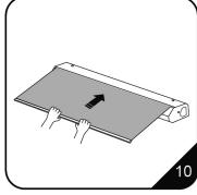
10. Carefully allow the graphic to recoil into the base unit (it may be useful to have an assistant hold the base steady).
