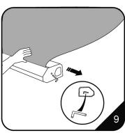
9. Peel off the cover, remove the screw underneath the chrome end of the base and detach. Then, with the graphic held firmly, carefully pull out the retaining pin, then put it into the cover.
