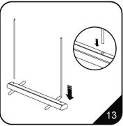
13. The bottom of the assembled pole slides into the round socket in the base unit.
