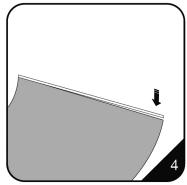
4. Paste aluminium bars one by one upon the upper and down edges of the graphic.
