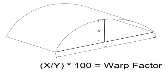
The maximum allowed warp percentage is 2.5, values above this will result in the board being identified as non-conforming and will require authorisation as to its suitability to meet customer's needs.
