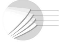
Clearcoat – Polyurethane Film - Polyurethane Adhesive - Acrylic PSA **Release Liner - Polyester**
