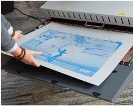
▲ The imaged plates are manually fed through the integrated finishing unit which dries the plates and bonds the liquid dots to the plate surface.
